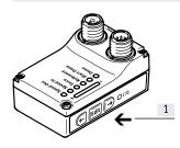
[1] Pushbutton actuators for parameterisation and control
